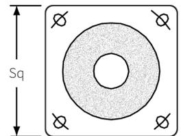
1C2 slotted base plate prestressed to pole
