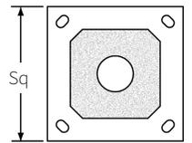
1C5 slotted base plate prestressed to pole
