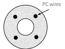
0C2 / 1C2 shaft cross section detail
