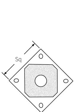
1C5 diamond pattern slotted base plate prestressed to pole
