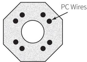
9CT Shaft Cross Section Detail
