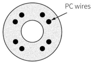
Shaft cross section detail
