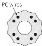
Shaft cross section detail
