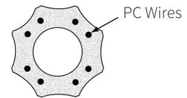
Shaft cross section detail
